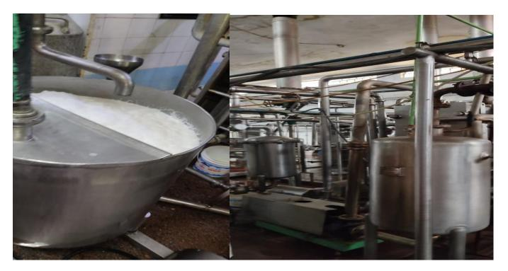
Milk being in the storage was processed into the equipment's so it gets processed into different phases of pasteurization and gets into the machine where packets are filled with different quantities of milk and then passed on to the storage place where the temperature would be 10 degrees Celsius. Finally the kettle of packets get transferred to the delivery to different places.
